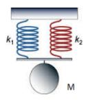
Question-4: Derive the equation of motion of the mechanical system shown below
